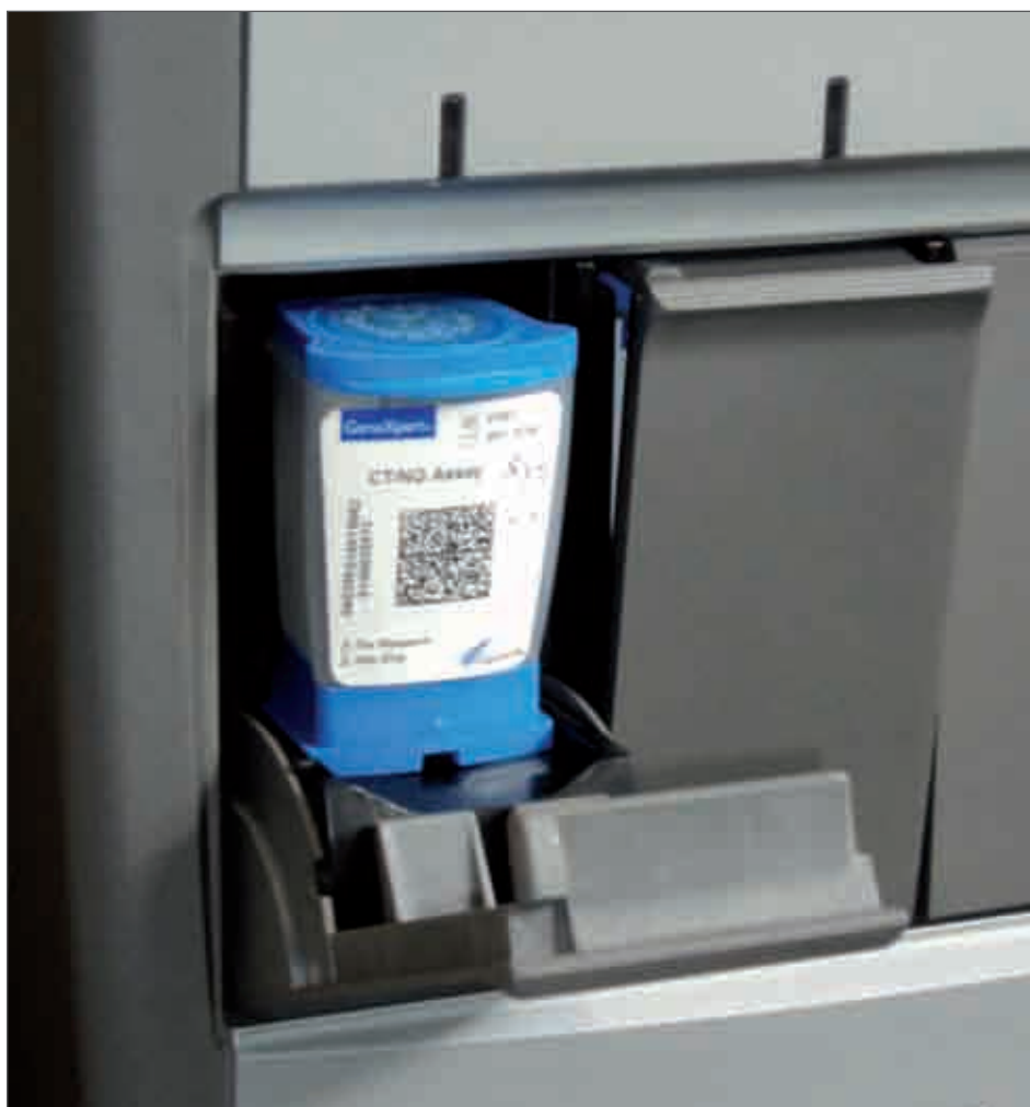
A test cartridge loaded into the Xpert machine, ready for testing.
